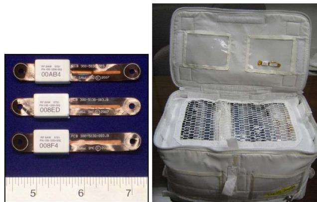
Figure 3: Flexible antenna RFID tags and crew bag with tagged items inside
