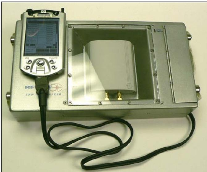
Figure 4: NASA version of RF SAW Model 704 Reader (shown with PDA)
