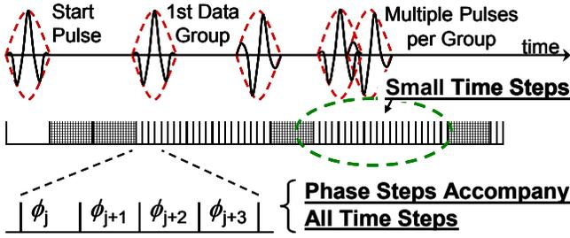
Figure 3: Global SAW Tag Data Encoding Example
