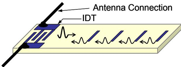
Figure 1: Schematic of a Typical SAW Tag
