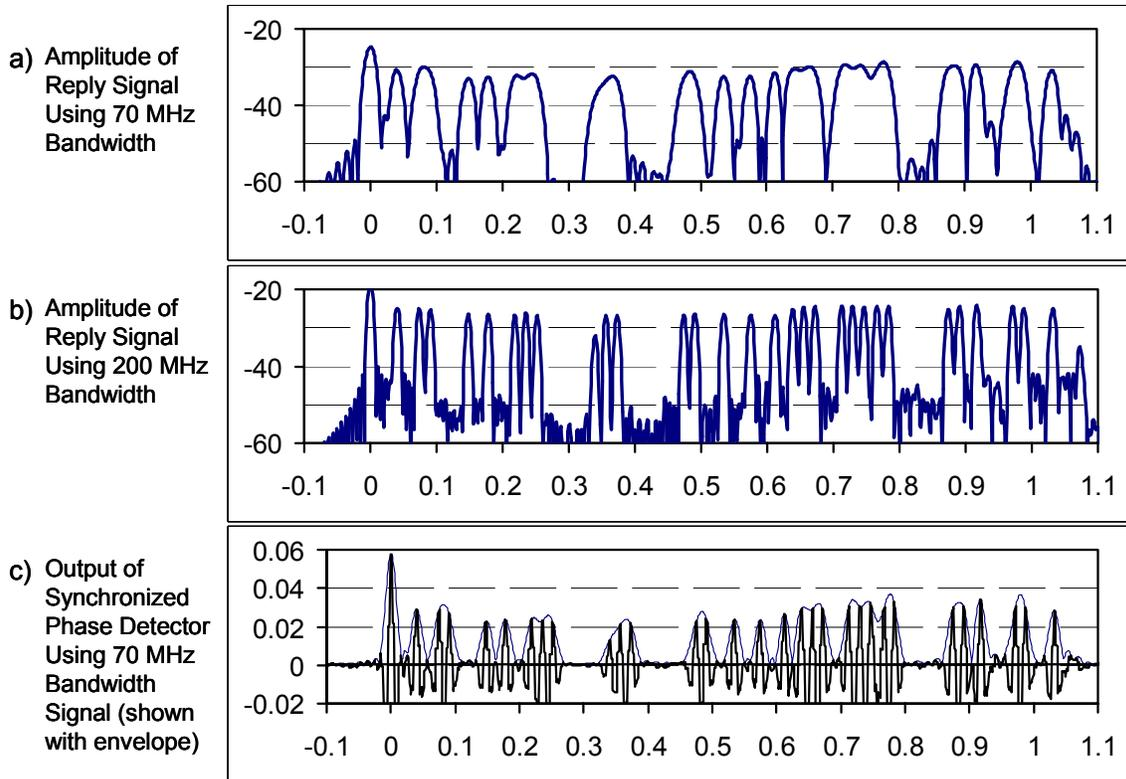
Figure 6: Pulse Response from 2.44 GHz Global SAW Tag with Pulses for Start, Stop, Synchronization, 64 Data Bits, and 16 Bit Error Detection. Uses Fundamental Mode Design on  $128^{\circ}$  LiNbO<sub>3</sub>
