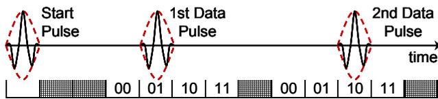
Figure 2: Data Encoding for an Existing SAW Tag
