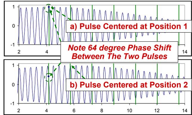
Figure 4: Phase Shift Between Two Adjacent Taps
